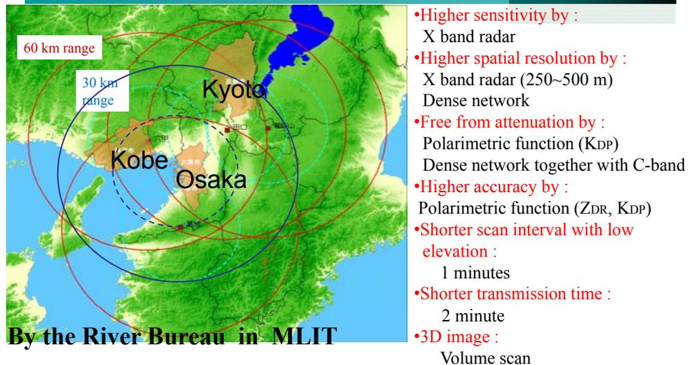
New operational networks by X band polarimetric Doppler radars are scheduled to be in operation in various urban areas in Japan before next April. Copyright 2009 by Eiichi Nakakita
