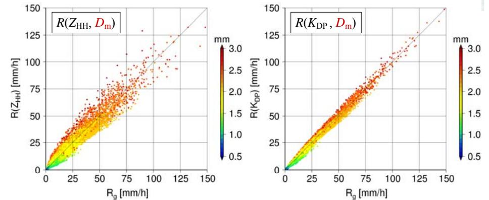
$$R(Z_{HH}, D_m) = \begin{cases} 3.49 \times 10^{-2} Z_{HH}^{0.724} & 0.0 \leq D_m < 1.0 \\ 7.72 \times 10^{-3} Z_{HH}^{0.852} & 1.0 \leq D_m < 1.5 \\ 3.39 \times 10^{-3} Z_{HH}^{0.878} & 1.5 \leq D_m < 2.0 \\ 3.13 \times 10^{-3} Z_{HH}^{0.867} & 2.0 \leq D_m < 2.5 \\ 1.60 \times 10^{-4} Z_{HH}^{1.083} & 2.5 \leq D_m < 3.0 \end{cases}$$
